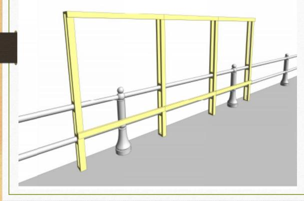
Temporary wooden frames are constructed snuggly around the boardwalk railing to use the structural integrity of the metal railing.
